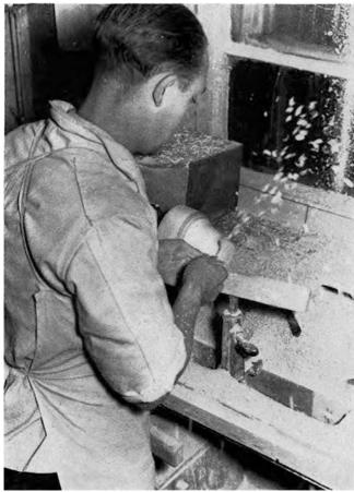
The "Turner" turns the cup or other round article on his lathe, after the thrower has finished his work, and makes it smooth externally, to give it the brilliant finish characteristic of Shelley China
