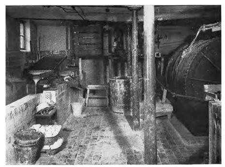
In the rotary Cylinder shown on the right, the ingredients are further ground and thoroughly mixed together. The resulting creamy mixture is called "slip," which is passed over the powerful magnet shown in the upper left corner to remove any metallic particles, into the trough, which is called the "Ark".
