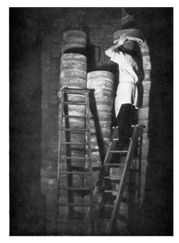
"Setting in " a Bisque Oven. The saggars filled with clay ware are stacked one on the other till the oven is filled. The ladder is known as the" horse," and the head placer as the "cod placer"
